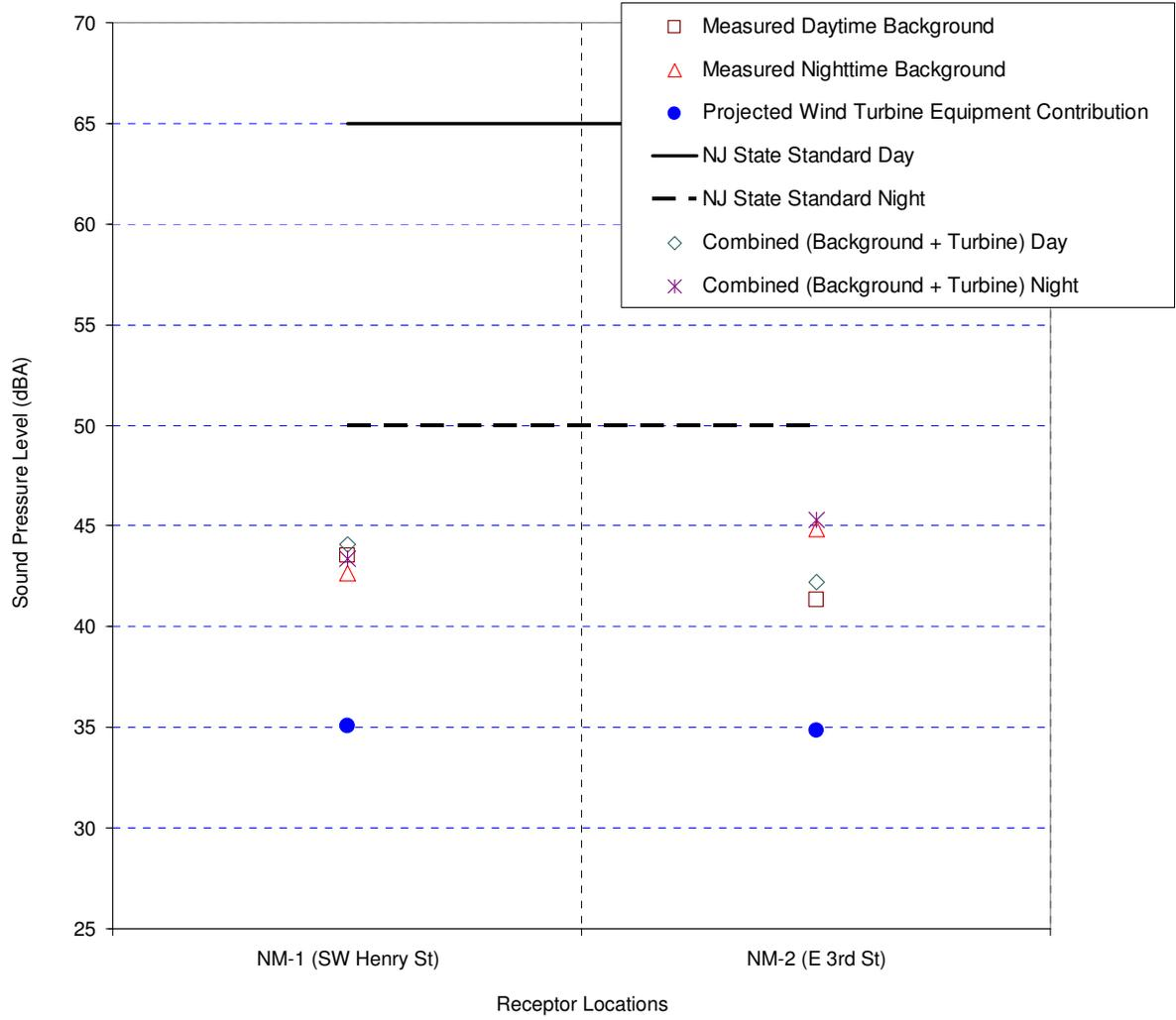
**Figure 5-6. BRSA Facility Projected Wind Turbine Sound-Levels
