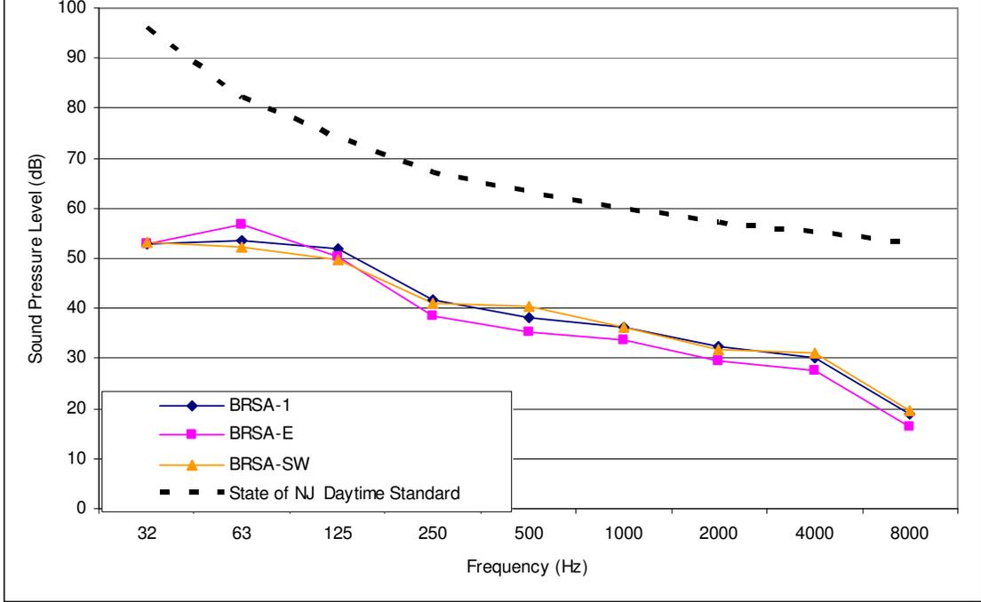
**Figure 4-5. Bayshore Regional Sewerage Authority Octave Band Sound-level Measurements (Nighttime)**
